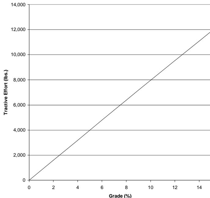
**Figure 2** shows the effect of grade on tractive effort required. For the example, a 2% grade would almost double the tractive effort required (1600 lbs. to overcome a 2% grade
