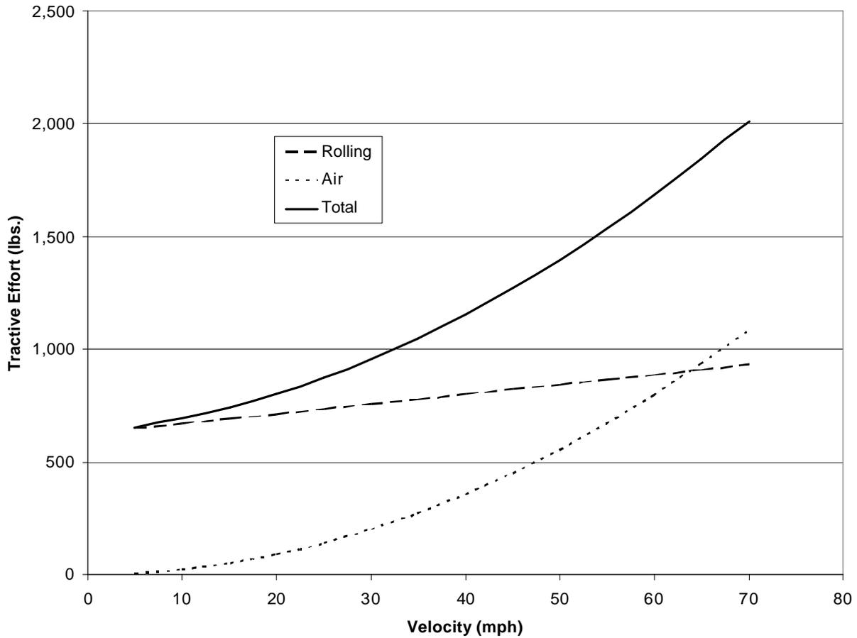
Rolling resistance is weight and road surface dependent with some change as velocity increases. Air resistance varies with the velocity squared and is minimal at lower speeds, but increases significantly after 20 mph and can become as significant as rolling resistance. Based on the tractive effort available in the highest gear (1987 lbs.), the top speed for this truck on level ground would be 70 mph; however, the impact of grade must be added to the values in **Figure 1**.
