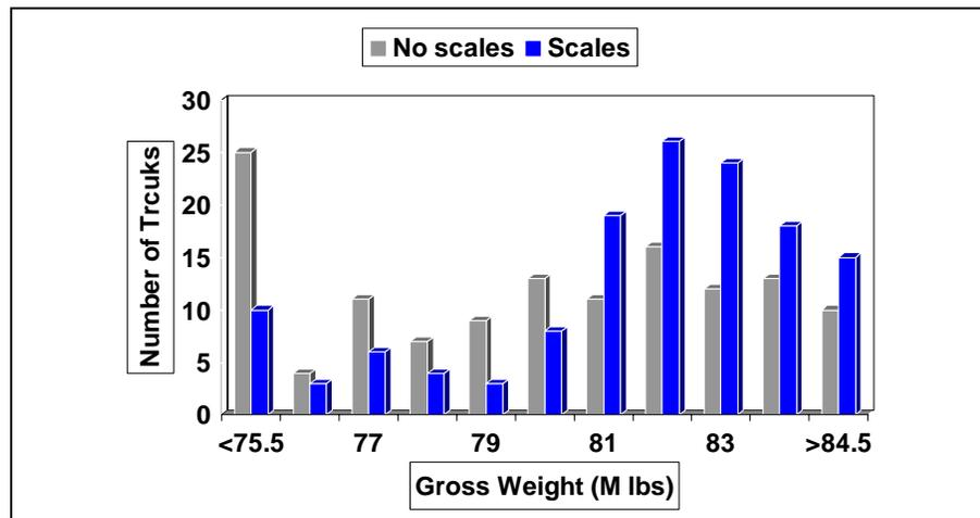
*Fig. 1: . Gross weight of trucks using scales versus trucks not using scales from locations where some in-woods scale use was observed. NOTE: Weight limit plus tolerance is 80,000 pounds in NC, SC, GA; 84,000 in MS, TX; 86,600 in LA; and 88,000 in AL.*
