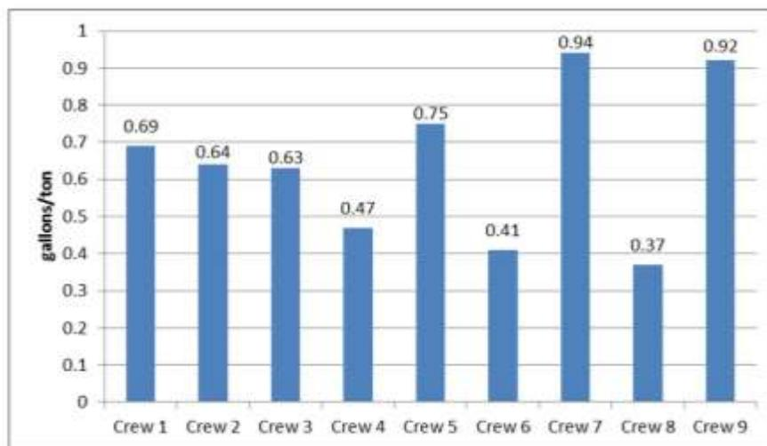
*Fig. 1: Average fuel consumption from individual tract data (ground-based systems).*
