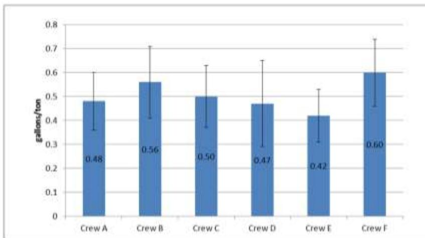
**Fig. 2:** Average fuel consumption from weekly data for the harvest of mostly treelength products processed at the landing. Error bars represent the 90% confidence interval for each crew.
